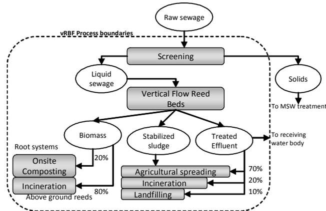
Fig. 2. Flow chart of the constructed wetland (vRBF) system
