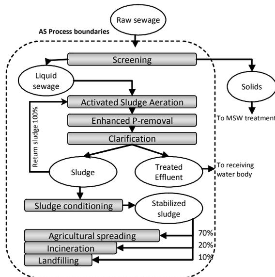
Fig. 3. Flow chart of the activated sludge system
