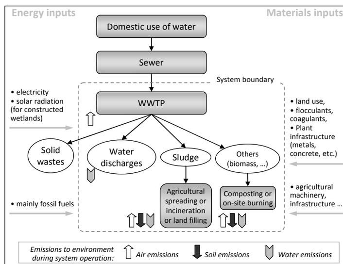
**Fig. 1: Flow chart of the wastewater system**
