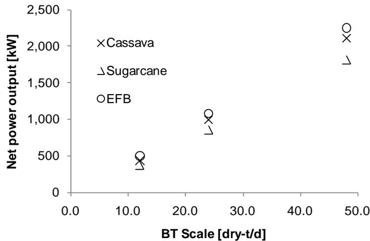
Fig.5: Net power output for BT scale (Bio-electricity case)
