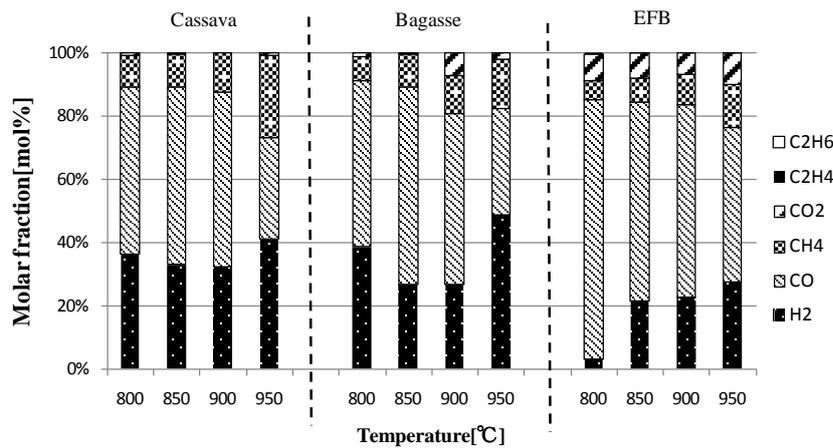
Fig.4: Results of steam reforming experiments
